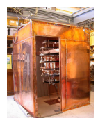
New 5 mT vertical system for in-vivo HP- ^3\text{He} lung NMR
