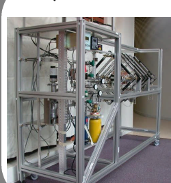
New 5 mT vertical system for in-vivo HP- ^3\text{He} lung NMR
